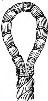
FIG. 90 B.—Flemish eye (complete).
